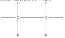
Due to presence of stable & strong C-F bonds, PTFE molecule possesses outstanding chemical inertness, high heat resistance & remarkable electrical insulation characteristics; in addition to excellent frictional properties.
